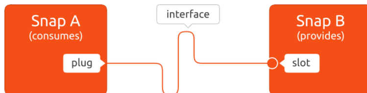
Figure 6.4 – Interface slot and plug
